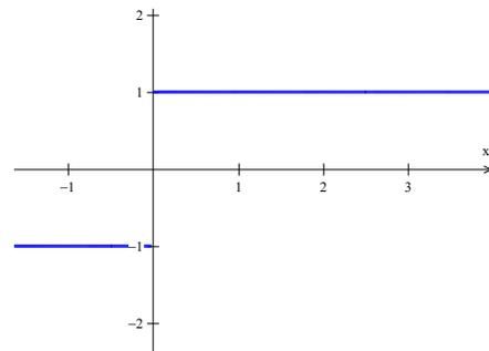
Figure 6 Bipolar step  $\frac{x}{|x|}$
