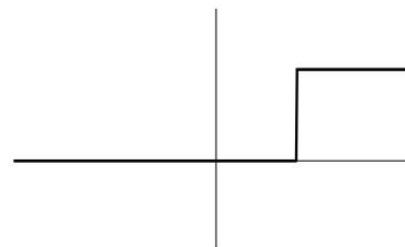
Figure 8 Delayed unit step  $u(x-a)$
