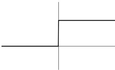
Figure 7 Unit Step  $u(x) = \frac{1}{2} \left\{ \frac{x}{|x|} + 1 \right\}$
