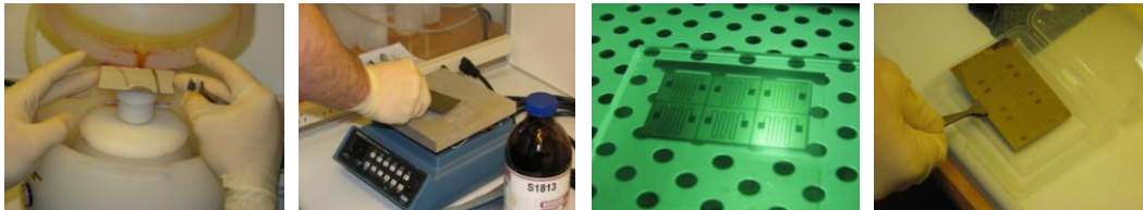
Figure 7. Fabrication of an RTD using photolithography.
