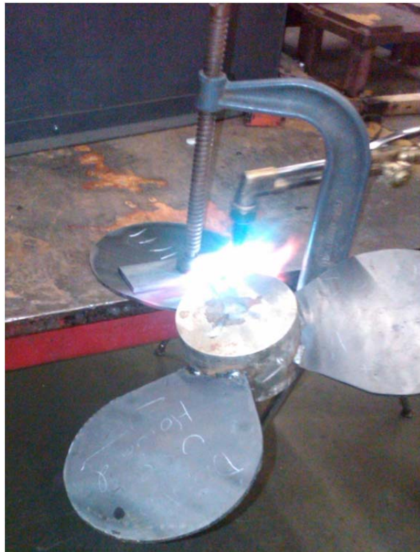
Figure 16: Fabrication of a New Blade Design for Hydro-kinetic Testing (Heating Blades to Bend Pitch Angle)
