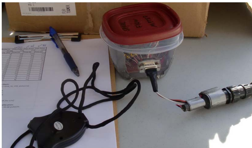
Figure 9: Custom Built Low-Cost Reader for the Swoffer Velocity Sensor
