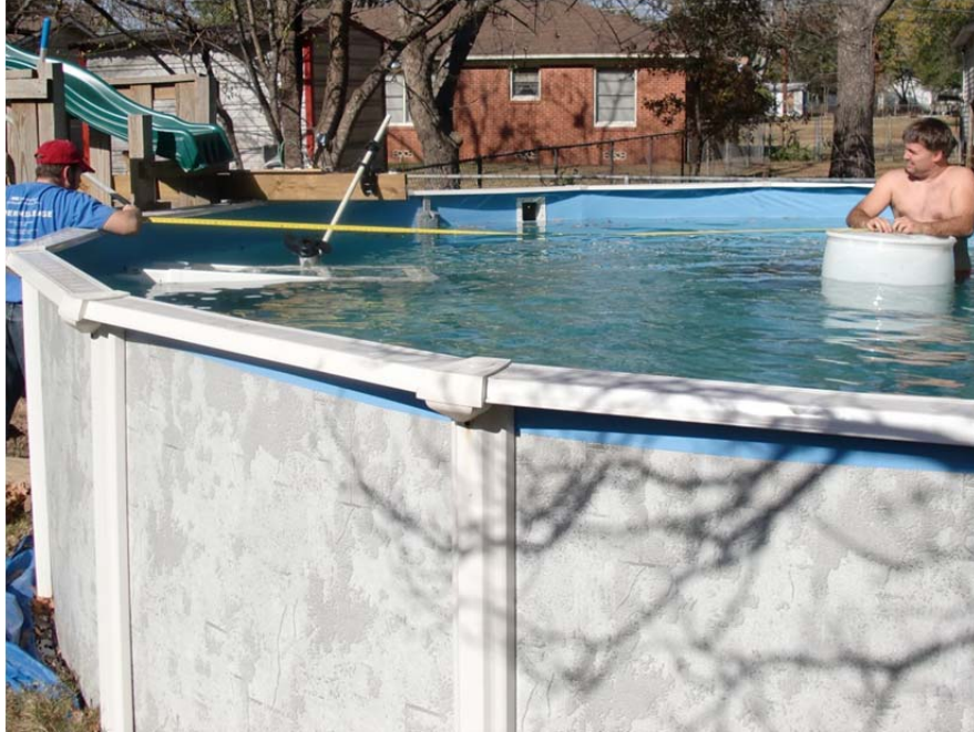
Figure 6: 24ft Pool and Vortex Suppression Barrel Being Centered
