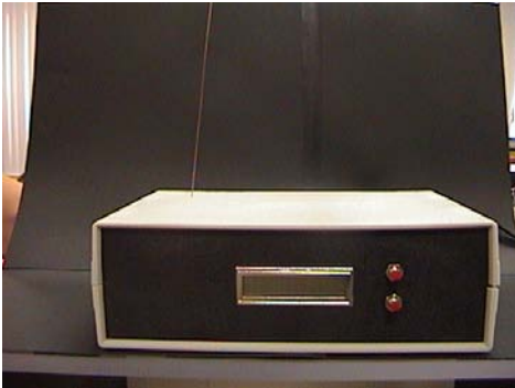
Fig. 8: The front layout of the case holds a LCD screen and two buttons
