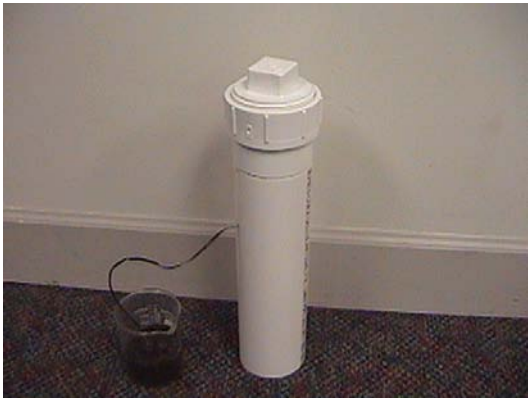
Fig. 5: Sensor case of 3" diameter PVC
