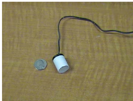
Fig. 1: A gypsum block for moisture reading
