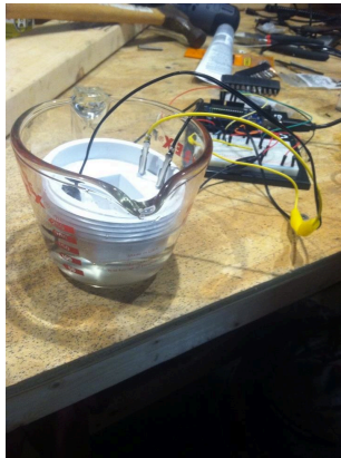
Figure 3: Arduino-based “Riffle-ito” water conductivity meter
