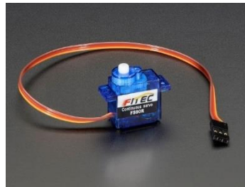
Figure 11: Servos used in the APD
