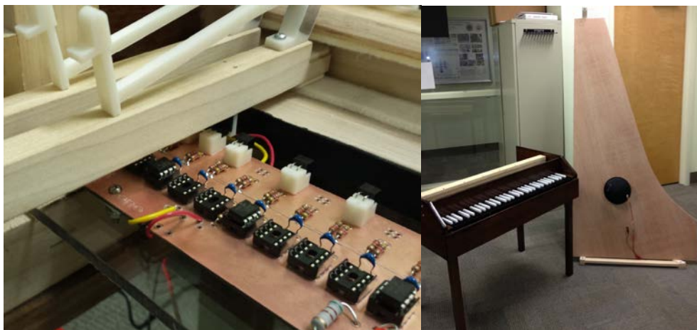
Figure 10 Mounted and Partially Populated Control Board (left); Full-Scale Soundboard and Electronic Fortepiano (right)
