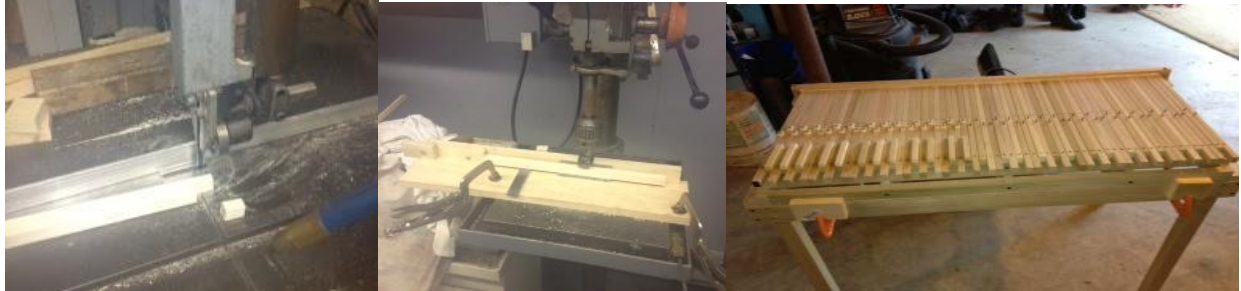
Figure 5. Cutting of the Keys (left); Key Pivot Hole Drilling Jig (middle); Keybox with all Key Blanks, Horseshoes, and Frame(right)
