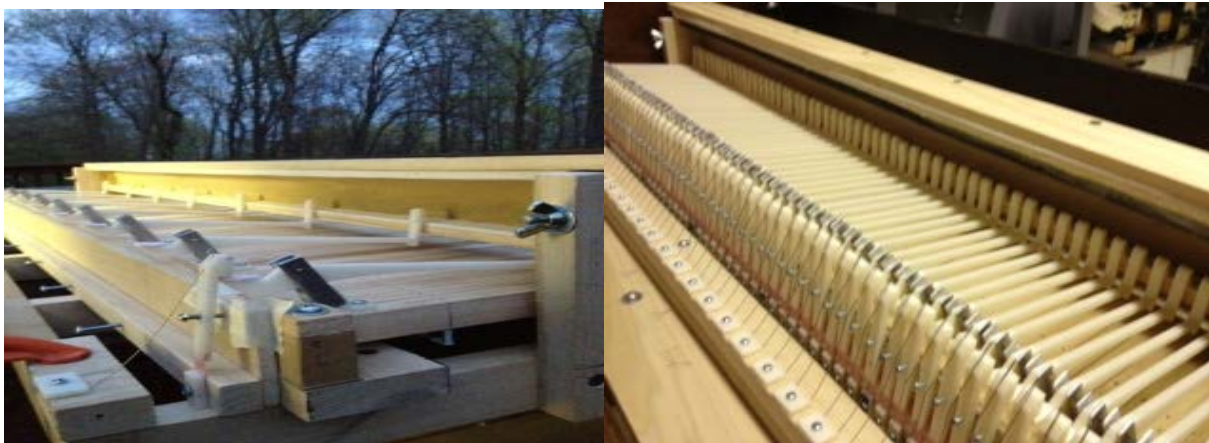
Figure 6 Completed keyboard internals (left); Hammer head resting on felt (right)
