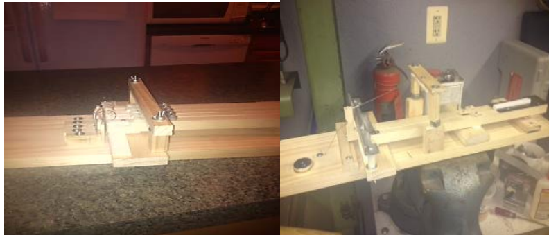
Figure 2 Coil Spring Key Return (left); Dual Leaf Style Spring Key Return (right)
