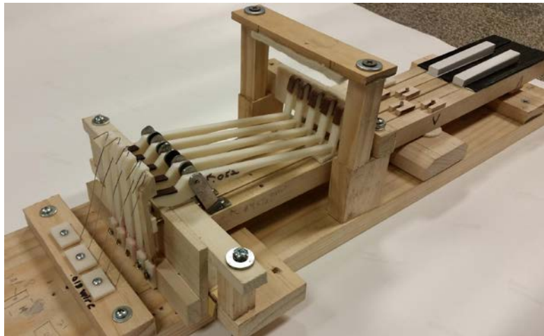
Figure 4 Key Prototype with 3D Printed Hammers and escapement system (Top);
