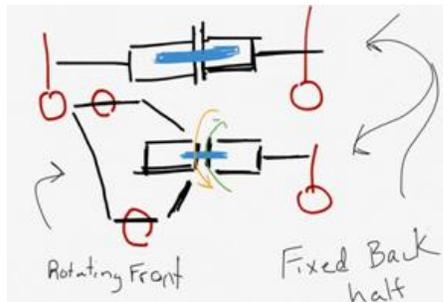
Figure 3, Use of Swiveling Center Drum Concept
