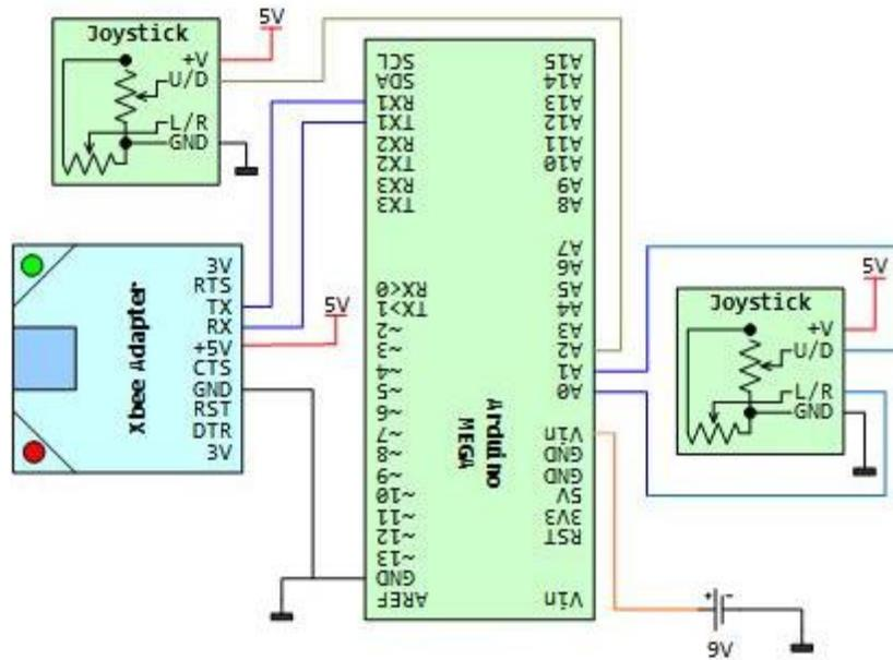
Figure 7 Twisted Sister Rover Remote Control Unit
