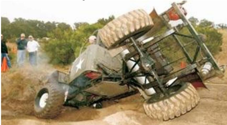
Figure 1. Articulating Chassis. (courtesy FourWheeler.com<sup>6</sup>)
