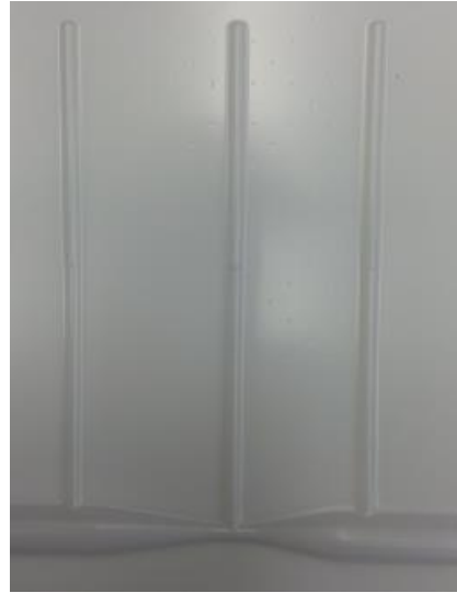
Figure 4. PETG sheet upon being removed from the vacuum former.
