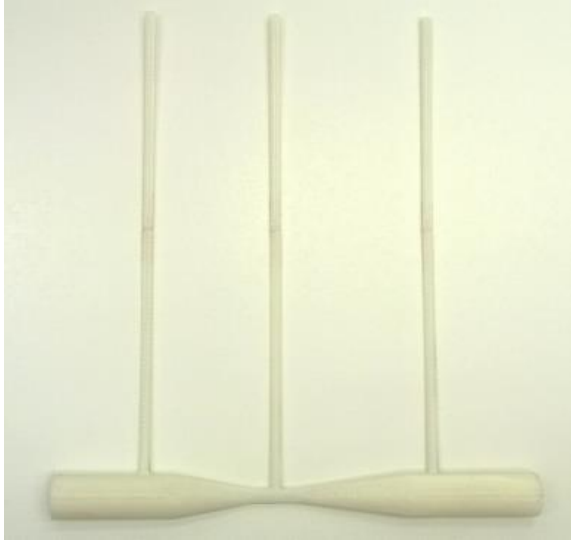
Figure 3. ABS plastic printout of the Venturi nozzle as taken from the 3-D printer.
