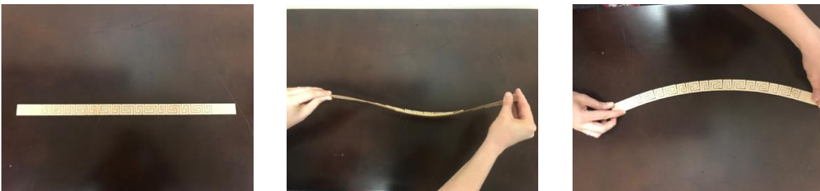
Figure 6: 1 of 30 additional beams featuring the living hinge pattern used in the project from Figure 5
