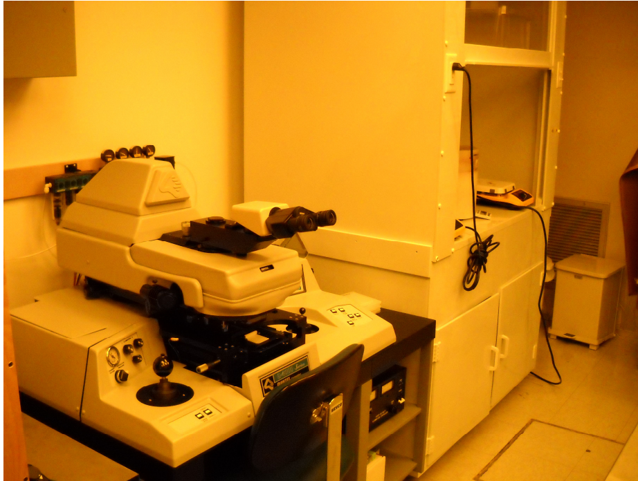
Figure 3: USNA Class 10,000 Cleanroom with View of the Mask Aligner
