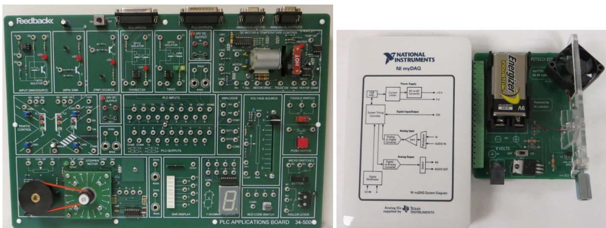
Figure 1: (Left) PLC Trainer Board, (Right) NI myDAQ & Pitsco myVTOL
