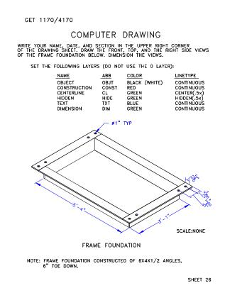
To make their working drawings students must create drawing layers utilizing abbreviations, colors and associated linetypes. In this drawing, as in the previous example, students improve their use of scales and layout skills. Students also become acquainted with angles as structural elements, and how they are used to create a machine foundation.
