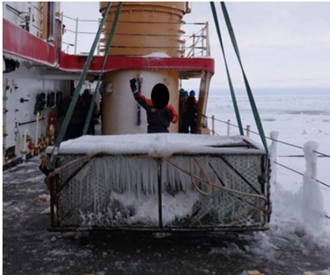
Figure 4. Results of freezing spray experiment by CGC Polar Star [1].
