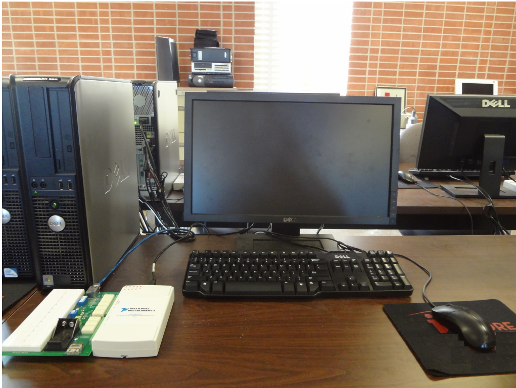
Figure 1: Individual workstation with National Instruments USB-6211 and protoboard.
