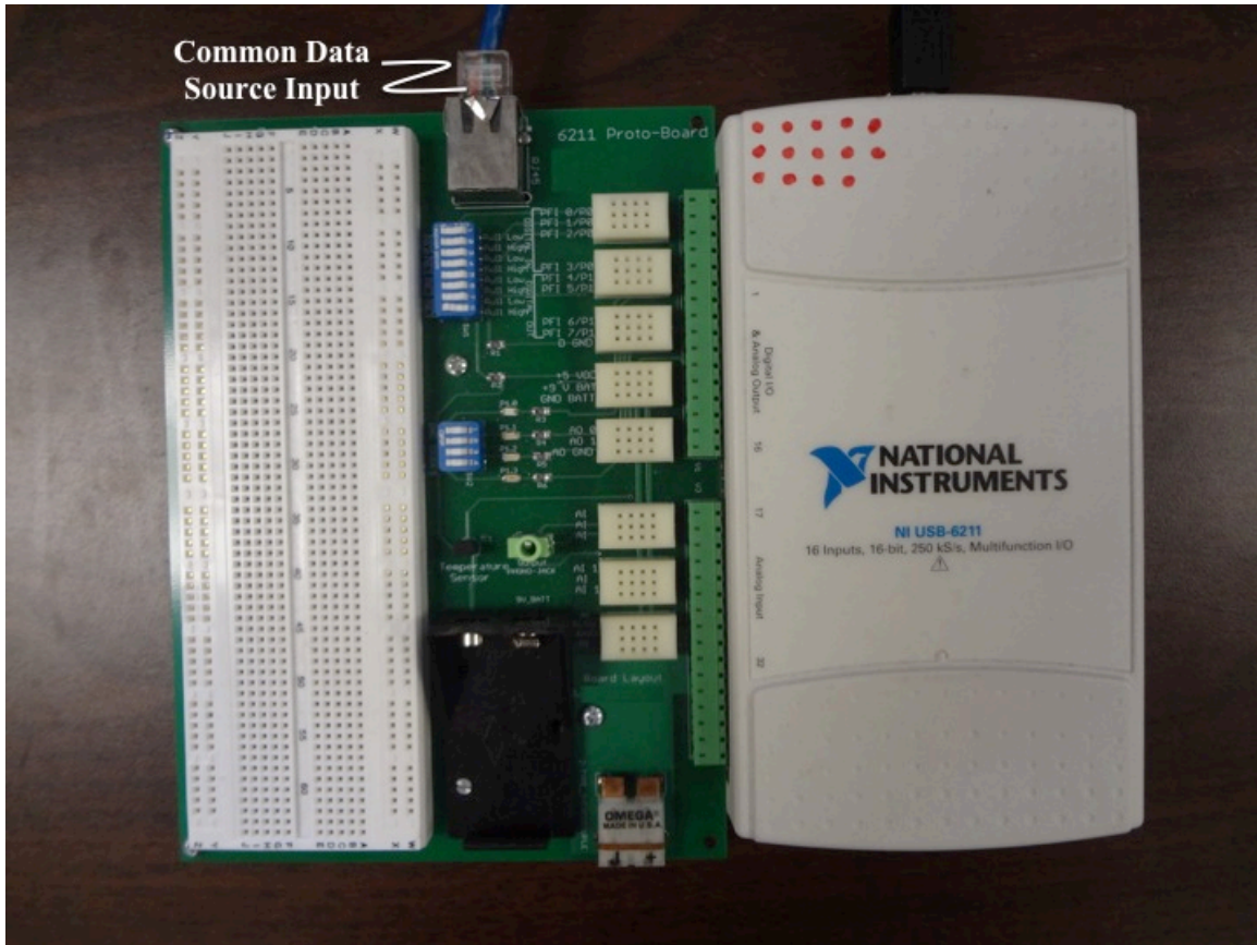
Figure 2: National Instruments USB-6211 data acquisition with attached protoboard, showing the common data source connection
