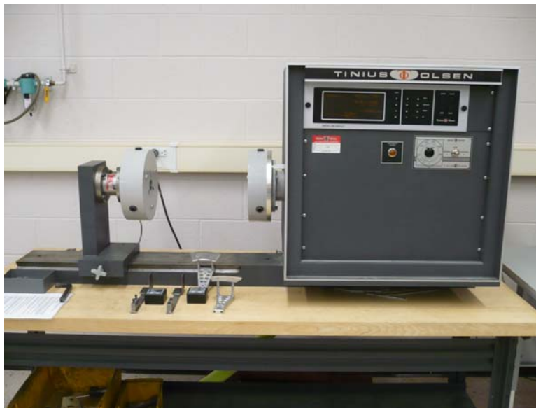
Figure 1: Tinius Olsen 10,000 in-lb Torsion Tester
