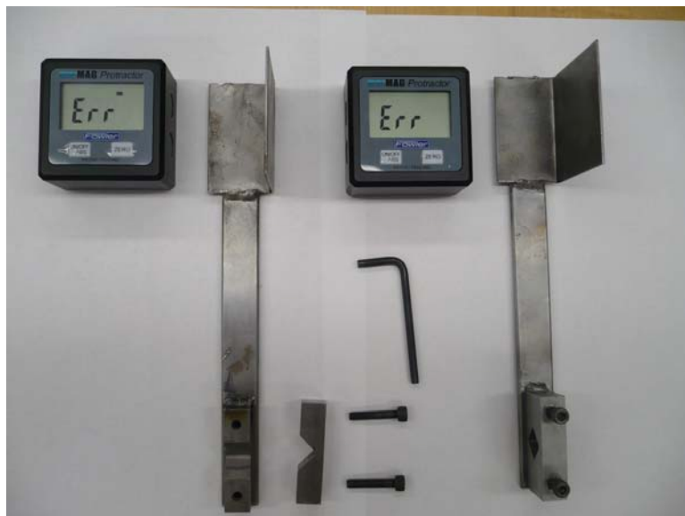
Figure 4: Inclinometers and Specimen Clamps
