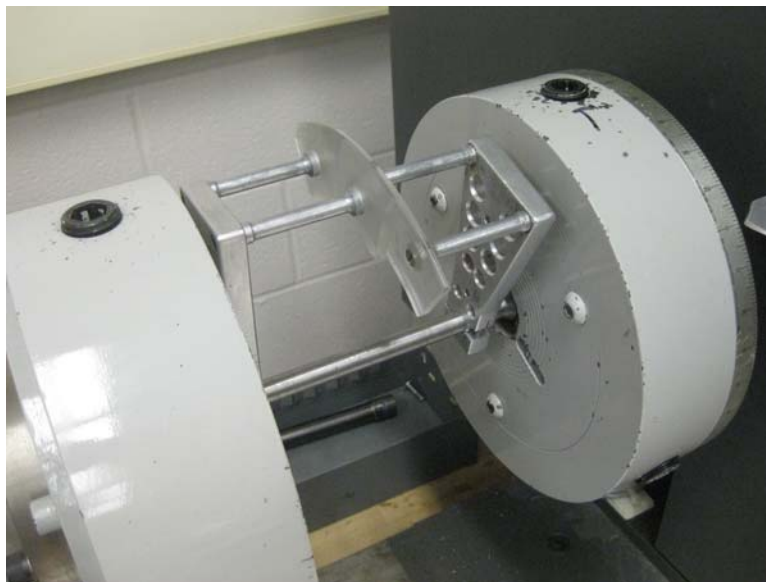
Figure 3: Troptometer mounted on specimen in Torsion Tester
