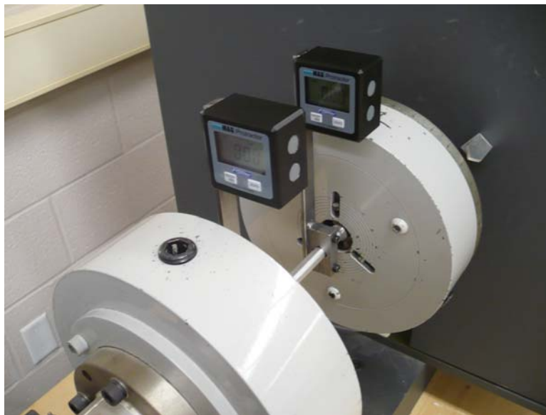
Figure 6: Inclinometers attached to specimen clamps in Torsion Tester
