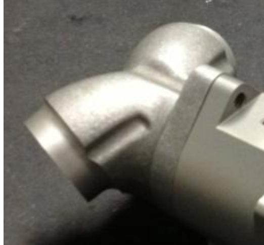
Figure 3. Commercial Common Intake Manifold Design.
