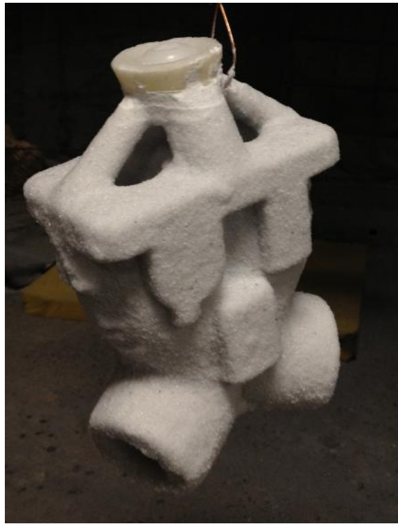
Figure 6. Hardened slurry on pattern.
