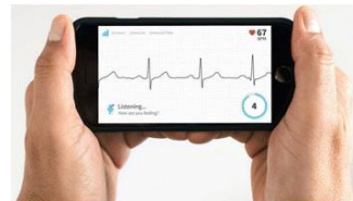
Figure 3: Alive Cor Kardia Mobile Device 6
