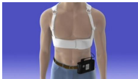
Figure 7: Wearable Cardioverter Defibrillator 11
