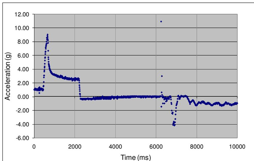
Figure 10. Actual model rocket accelerometer data plot
