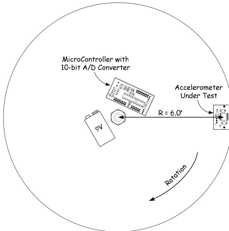
Figure 8. Centrifuge turntable PCB and battery mounting configuration
