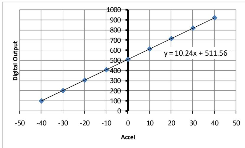
Figure 9. Plot of ±40g accelerometer centrifuge data
