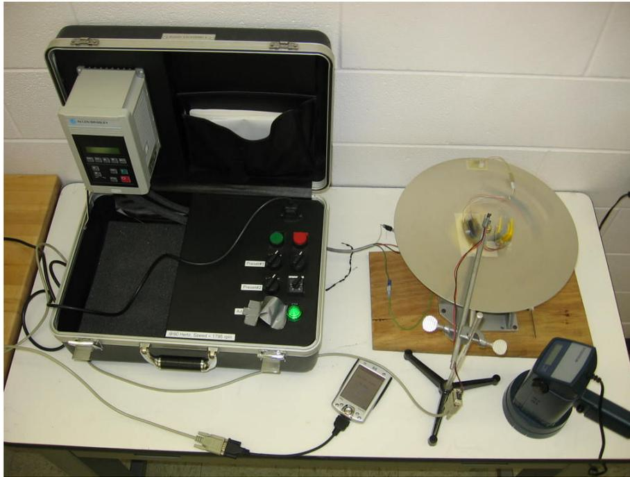
Figure 7. Variable frequency drive motor turntable centrifuge setup.
