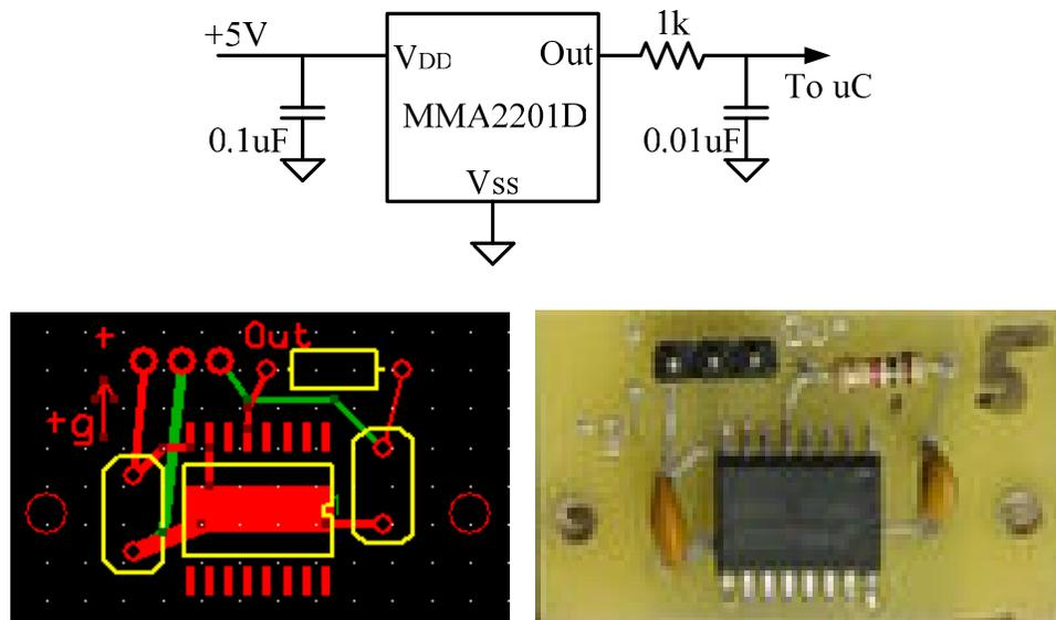
Figure 6. Accelerometer PCB schematic, layout, and photograph
