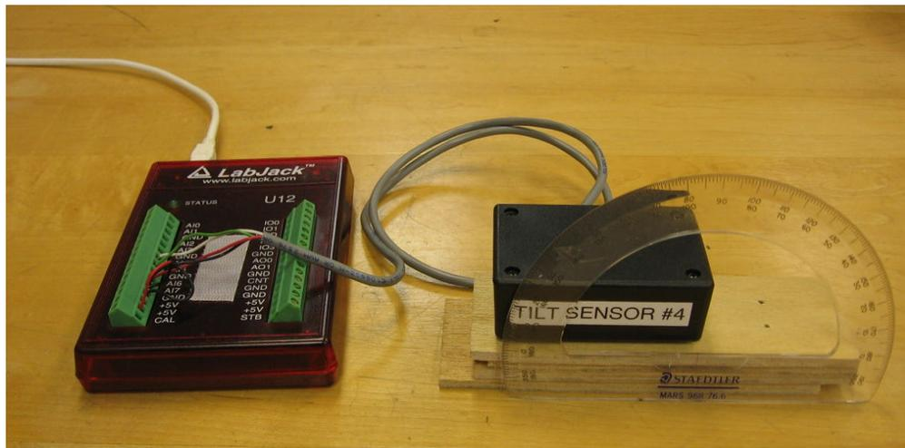
Figure 3.  $\pm 1.5g$  accelerometer inclinometer test setup
