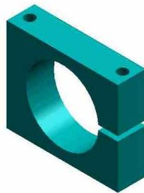
Figure 4. Rendered solid model of motor mount used in rapid prototyping exercise.
