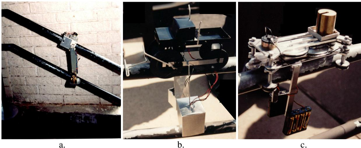
Figure 2. Rail Rider Solutions: a) worm driven rail rider with rubber wheels located illustrating the grade of the test rail, b) belt driven rail rider truck with apple-core wheels and c) belt driven, four-wheel drive design using magnetic drive wheels and carrying the 500-gram load.
