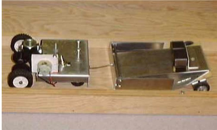
Figure 5. Tractor solution utilizing laminated paper RP motor mount and attached to advancing weight sled.
