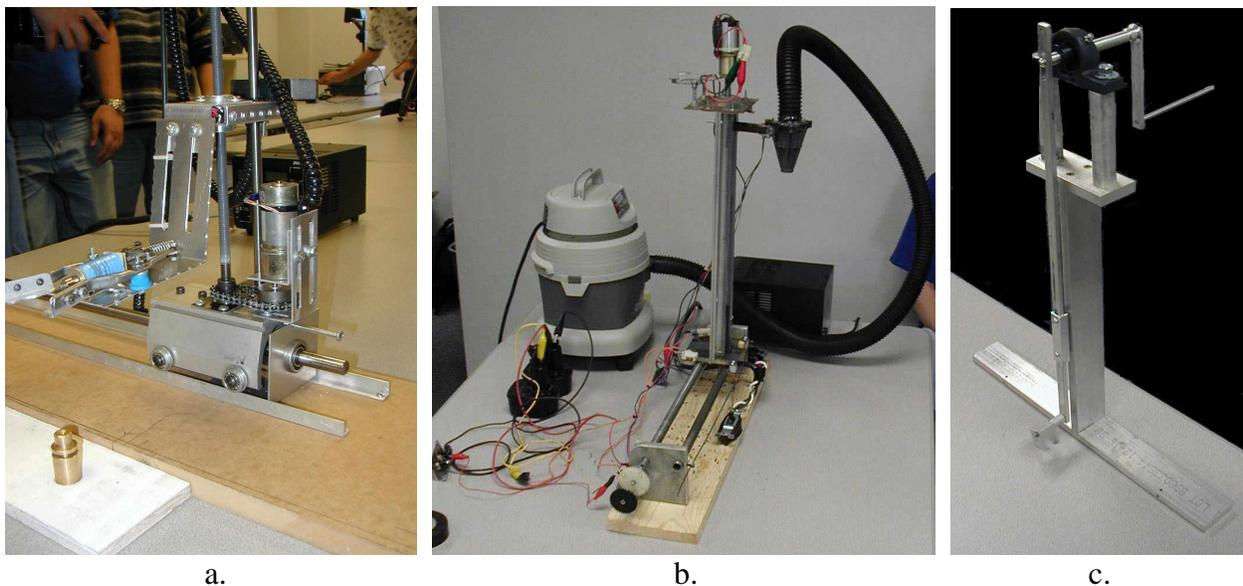
Figure 3. Solutions to the pick and place problem: a) a Cartesian solution using two-fingered, solenoid actuated gripper, b) a Cartesian solution using a vacuum based gripper and c) a rotary machine solution based on work cell / part geometry, utilizing a C-channel gripping device and hand-crank operation.
