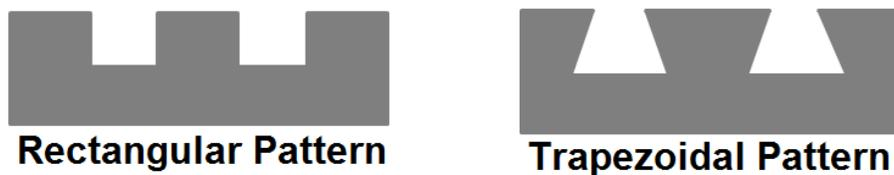
**Figure 1.** Schematic representation of die micro-geometries in the shapes of rectangular (left) and trapezoidal (right) features.
