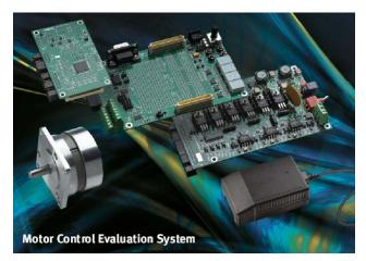
Figure 1: NEC Brushless Motor Control System
