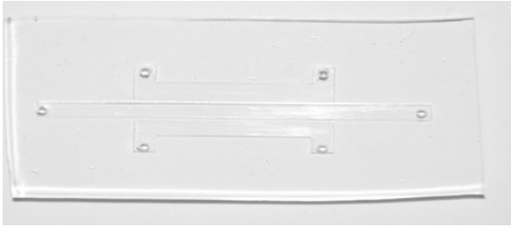
Fig. 4. Test of PDMS microfluidic device fabricated by replica molding of a Scotch-tape master. A) Image of a microfluidic device consisting of three independently-addressable microchannels. B) Microchannels filled with red or blue ink.
