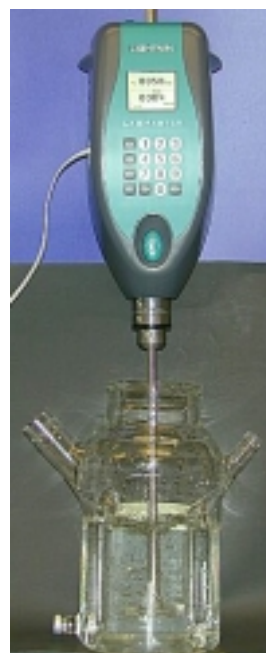
Figure 1: Mixer and 2 L Reactor
