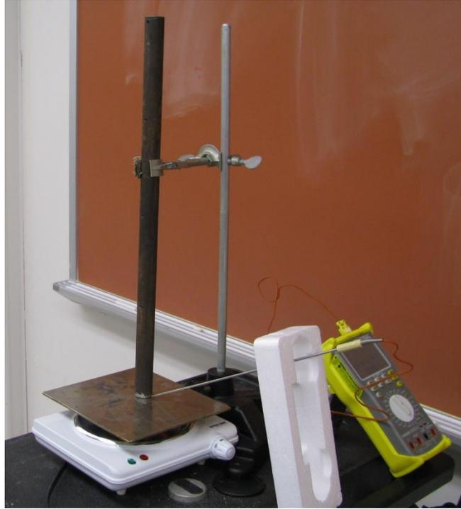
Figure 2: Conduction experimental setup
