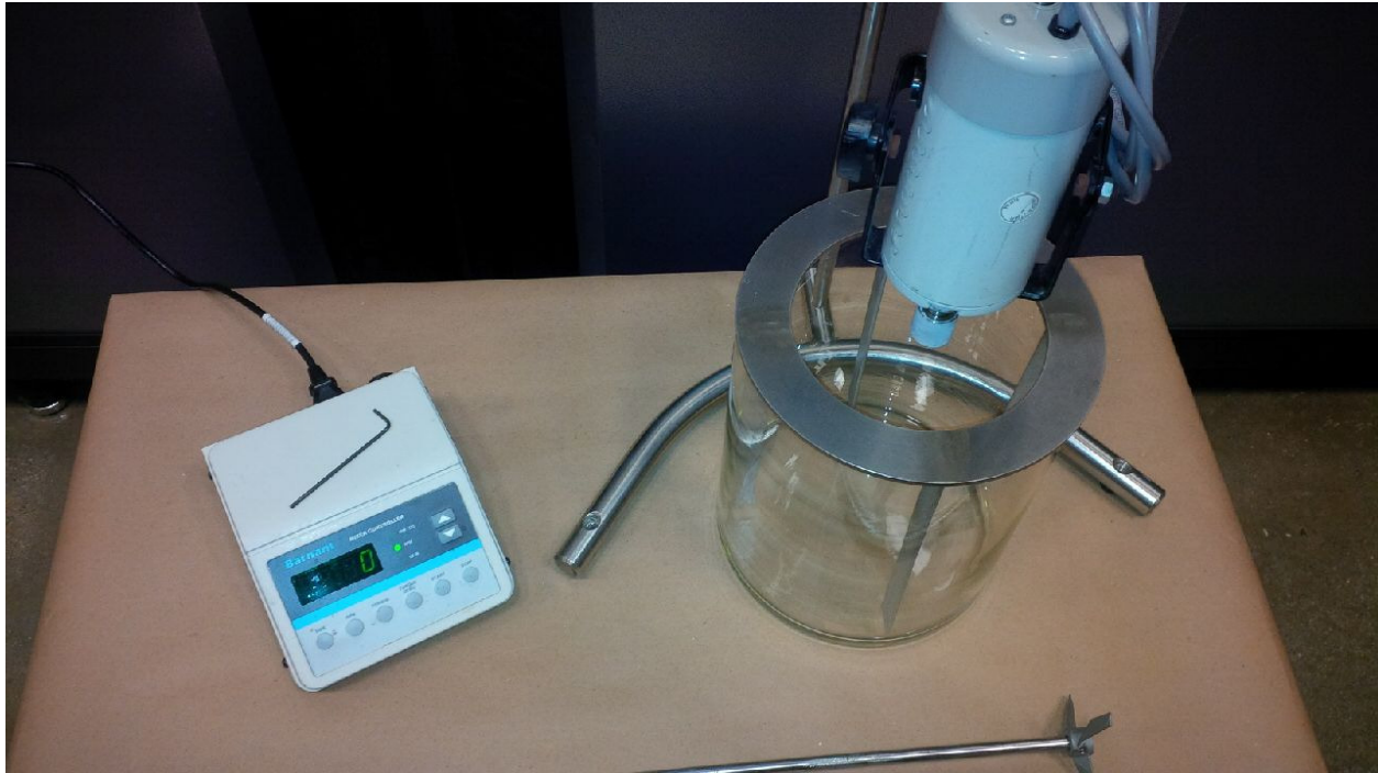
Figure 1: Vessel, baffles, motor and speed controller
