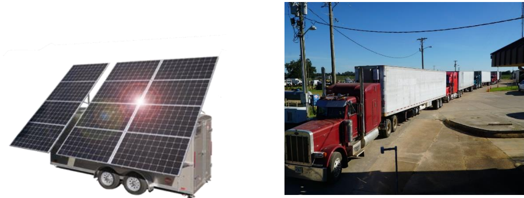
Figure 1. Commercially available mobile solar PV trailers (a) MS-325 7.2 kW rated, 35kWh battery capacity, 12 PV panels (24 kWh/day) [7], (b) FL-Escambia River Electric Cooperative (EREC) bunk trailers for disaster relief efforts [6].
