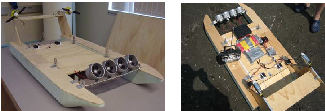
Fig. 3. PAR model under assembly and instrumented for initial testing. Length and beam of the model are approximately 115 and 60 cm.
