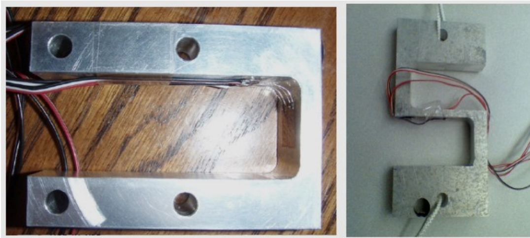
Figure 4: Load cell transducers designed and built by students with “C” and “S” shapes. The “C” design functions in two force ranges and the “S” design is similar to some commercially sold transducers.
