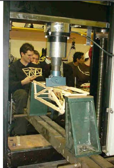
Figure 2. Loading frame utilised
