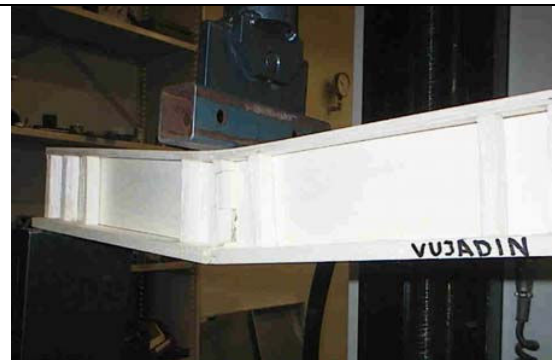
Figure 16. Tension flange failure
