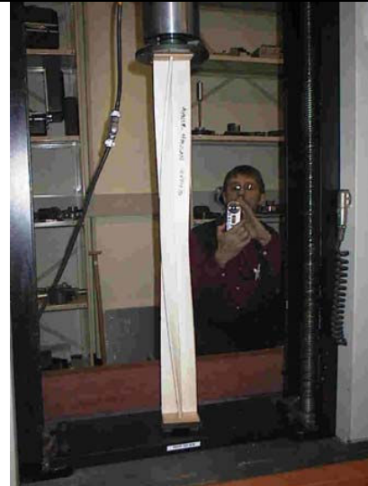
Figure 12. Torsional failure exhibited
