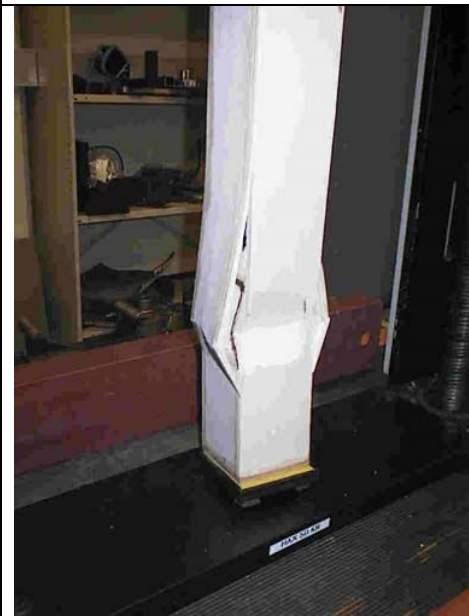
Figure 13. Crushing failure exhibited
