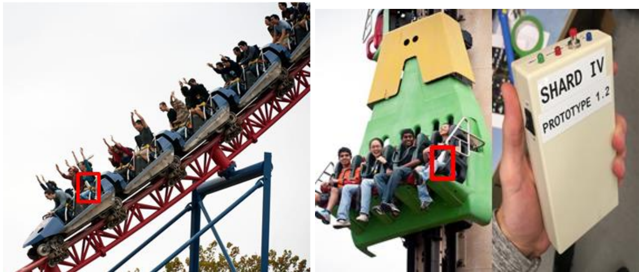
Figure 11: Six Flags trip: Students test their baroreceptor reflex at Six Flags Amusement Park by simultaneously measuring heart rate and acceleration. The SHARDs (Simultaneous Heartrate and Acceleration Recording Device) are indicated with the red box on the Superman roller coaster (left) and 140 ft free fall on VooDoo Drop (center). The fourth generation SHARD is shown at right.
