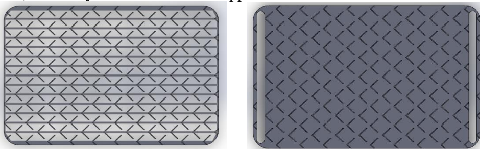
Figure 3: Comparison of the initial spacer design (left) and the newly developed design (right) with a full thick base.
