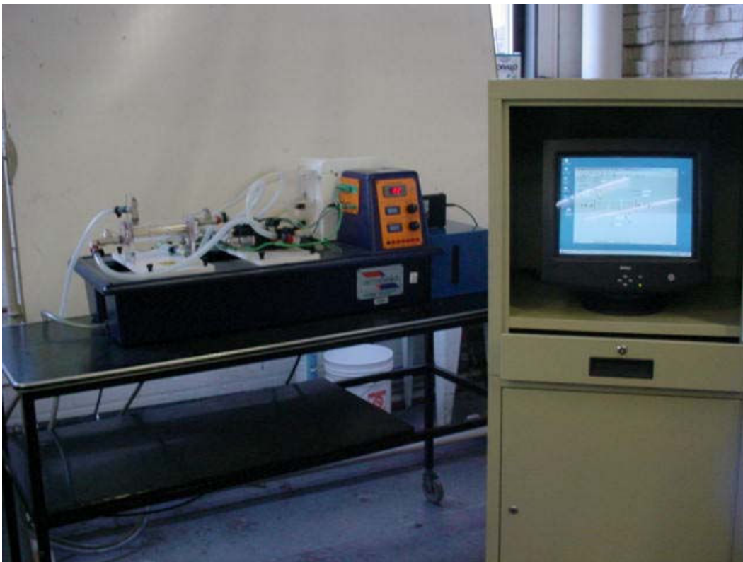
Fig. 6. Armfield heat exchanger unit.
