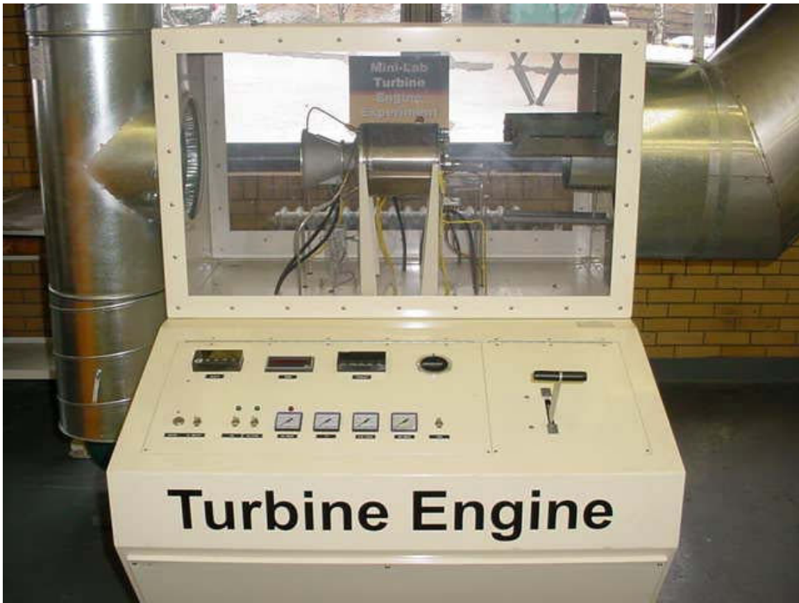
Fig. 4. Minilab jet engine from Turbine Technologies
