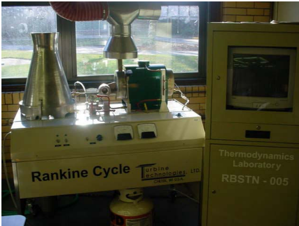
Fig. 2. Rankine Cycler micro steam turbine power plant from Turbine Technologies.
