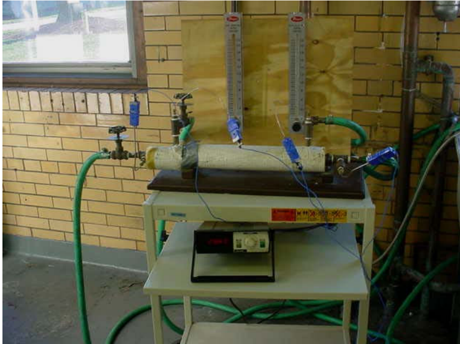
Fig. 5. Stainless still shell and tube heat exchanger.
