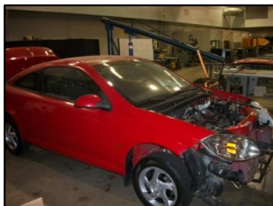
Figure 1: This photograph shows the 2008 Pontiac G5 used in BEV conversion. The 5-speed transmission was left in the vehicle to better match driving demands.
