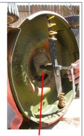
Maximum shear stress due to torsion will occur on the outside surface of the part of the shaft with the smallest radius
