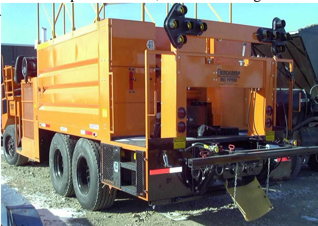
Figure 1: Paver operator's platform
