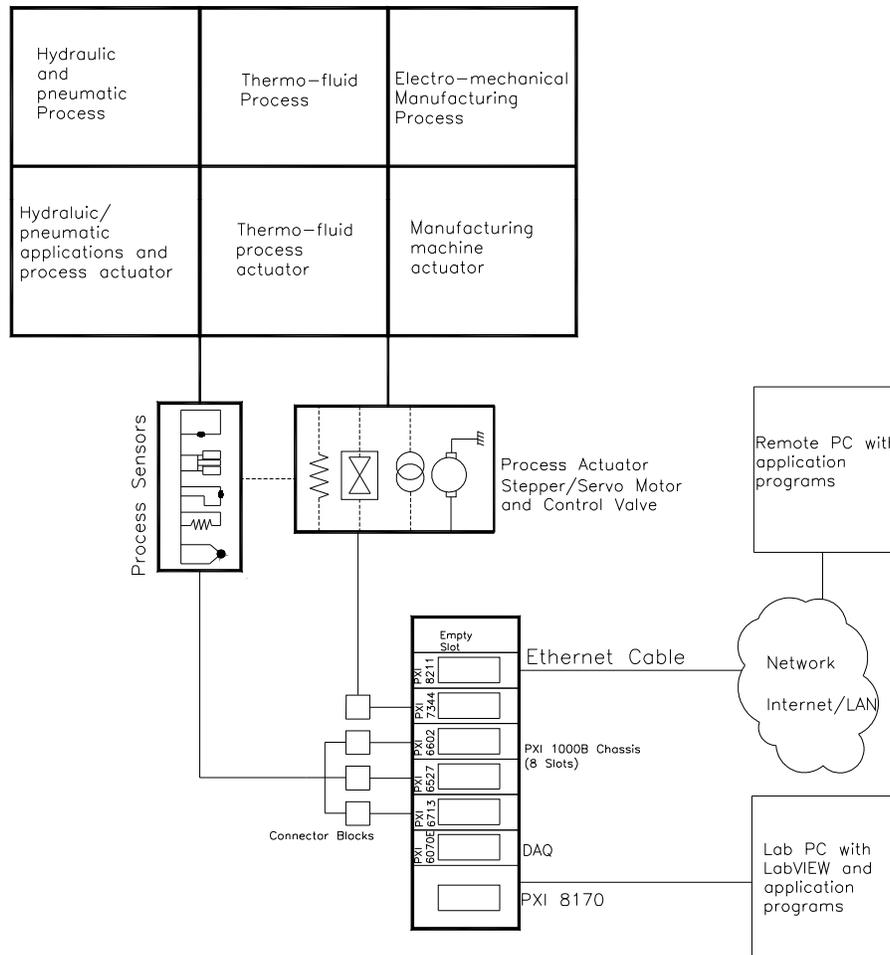
Figure 2. Layout of thermo-fluid laboratory
