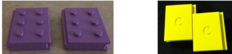
Figure 2. Braille tiles with dove-tail slots [6]
