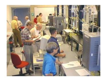
Day five's experiment was "Catalytic Oxidation of Volatile Organic Compunds (VOCs)". This experiment used a tube furnace with a palladium catalyst similar to the catalytic converter in an automobile. The objectives of the experiment were to determine the reaction kinetics of propane oxidation by varying the propane concentration and reaction temperature. Process streams were analyzed on-line with an FTIR.
