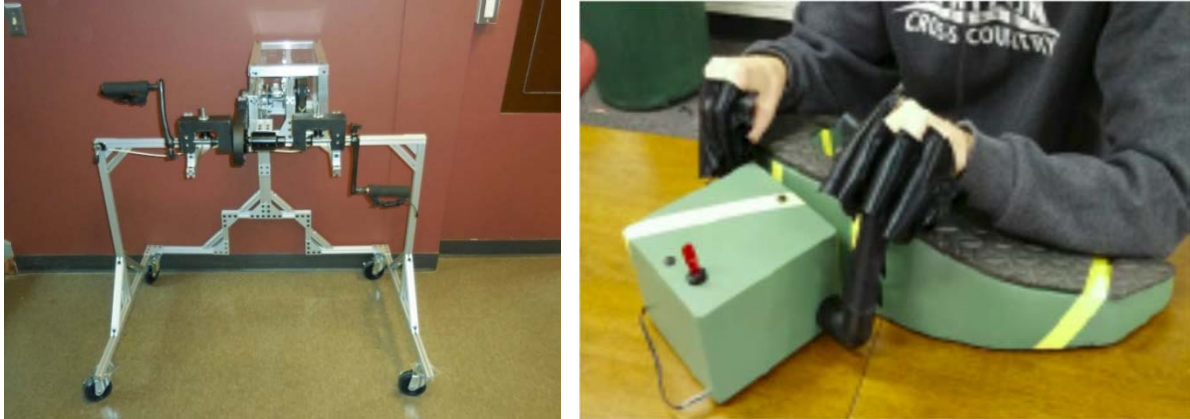
Figure 1: The collaborative project resulted in the development of two rehabilitation devices that allowed the clients to exercise upper body or hand muscles. Student teams must address client's feedback which is why the device was painted green with a yellow stripe.
