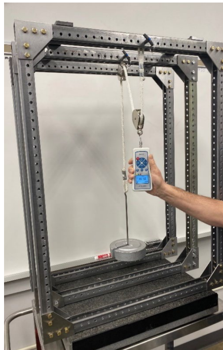
Figure 8. Example of hands-on application for the equilibrium of pulley assembly
