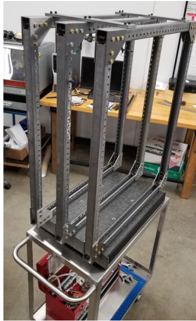
Figure 1. Developed moveable table for hands-on application in statics
