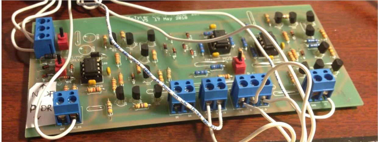
Fig. 3. Completed curve tracer connected to a myDAQ and to a test MOSFET (not shown). Connections to circuit terminals mentioned in the text (e.g., VCE\_DS) are made at the screw-type terminal blocks at the periphery of the circuit board.
