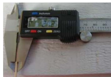
Fig. 5 A digital caliper with micrometer accuracy.
