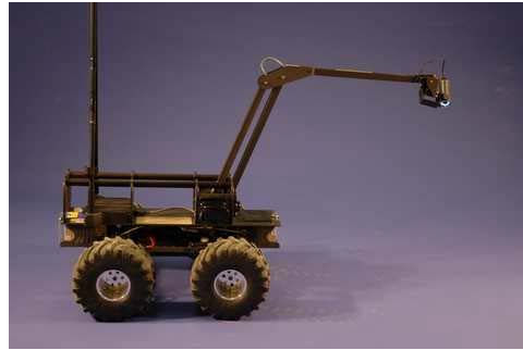
Figure 3. MARCbot-N small robot vehicle with 18" wheel base
