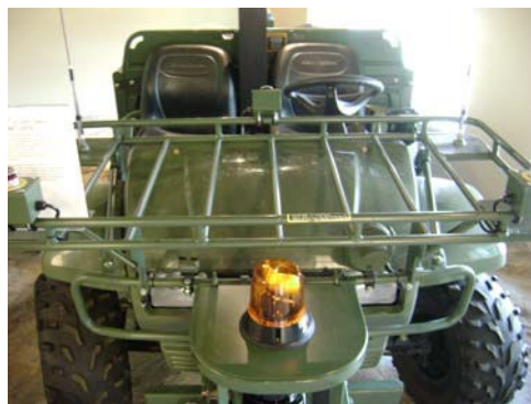
Figure 2 - R-Gator used at MSFC to simulate large surface vehicle
