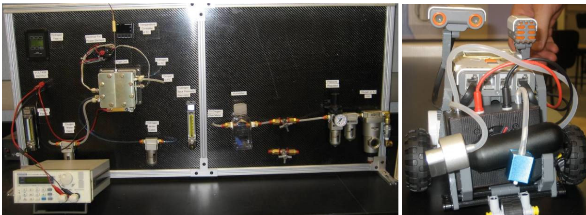
Figure 4. CSULA built fuel cell test stand with a 25 cm 2 fuel cell (left). Lego MindStorm robot powered by a Horizon H-20 fuel cell (right)
