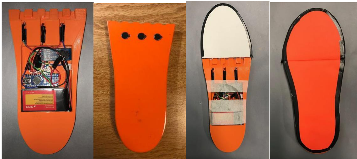
Figure 5: Physical Electronic Setup of Insole without Foam (first and second) and With Foam (third and fourth)
