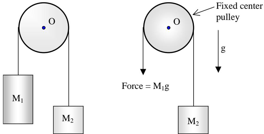
**Figure 2 – Schematic of contrasting dynamic systems**
