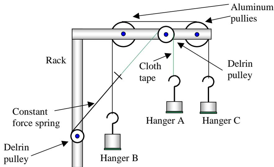
**Figure 3 – Demonstration set-up for mass-weight concept**
