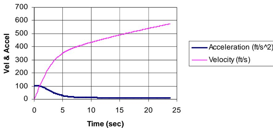
**Figure 7 – Rocket velocity and acceleration**
