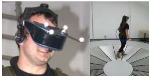
Fig. 4. Head Mounted Display and omnidirectional floor of the Virtual Theatre
