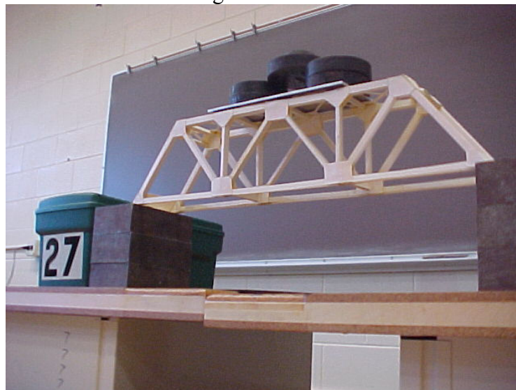
Figure 1: A successful bridge resisting the probabilistic design load.
