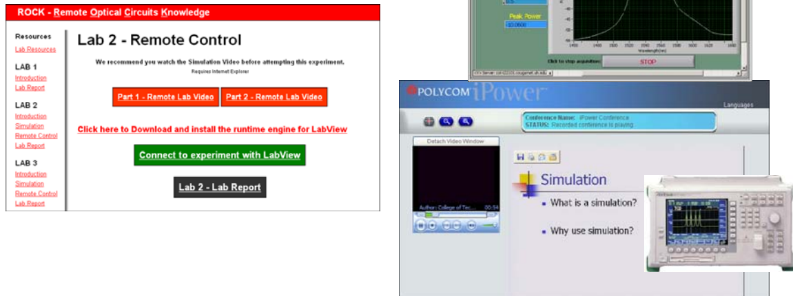
Figure 6. Many aspects of the experiment have been put together in this figure to demonstrate the access mechanism as well as emphasize the complicated media requirements in a virtual experiment. The orientation video screen, optical spectrum analyzer picture and spectrum screen and the web site links have been displayed.
